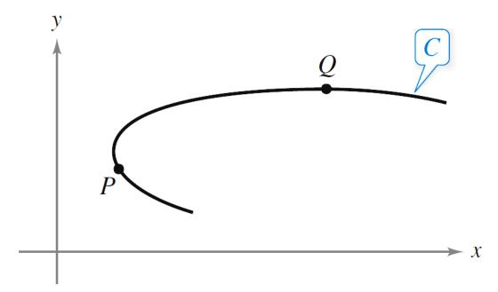
You can calculate curvature by calculating the magnitude of the rate of change of the unit tangent vector **T** with respect to the arc length *s*.
