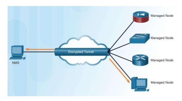
SNMPv3 authenticates and encrypts packets over the network to provide secure access to devices.
