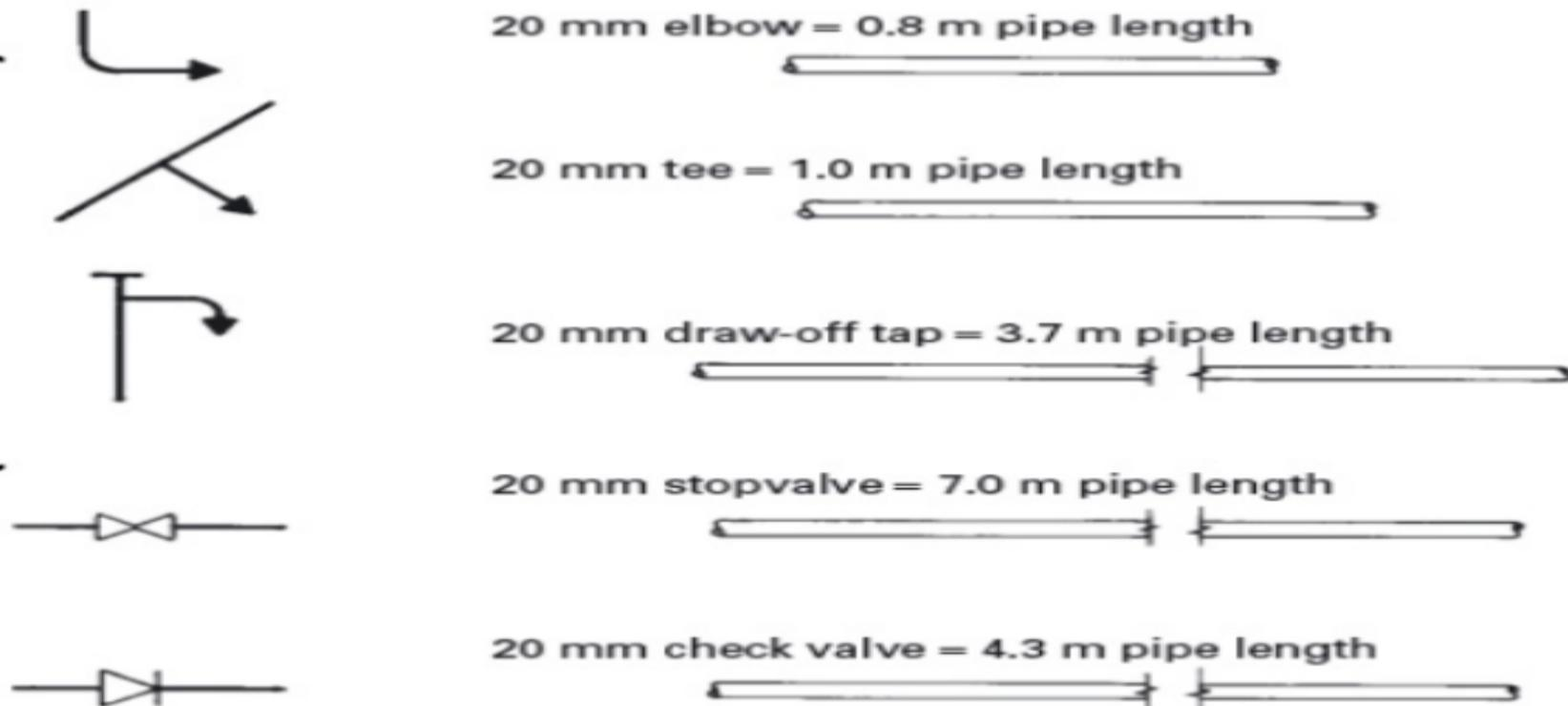
Table 1.9 Equivalent pipe lengths (copper, stainless steel and plastics)
